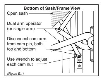
For sash adjustment, unlock and open sash. Use a flat head screwdriver to remove arm from each cam nut located on top and bottom hinge track. Use a crescent wrench to slightly rotate each cam nut a 1/16" to the exterior or 1/32" to the interior. (Figure E.1)
