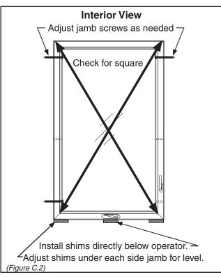
With sill shimmed and levelled, unlock sash and carefully open. Install (1) #8 x 2"
