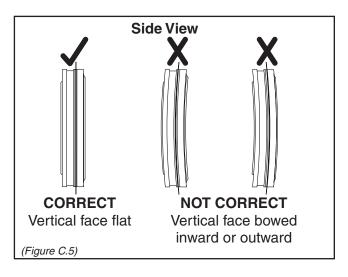
Check the plane of the window unit. Each vertical jamb side frame should be equal and parallel to the other. See illustration for equal and unequal plane. (Figure C.3)
