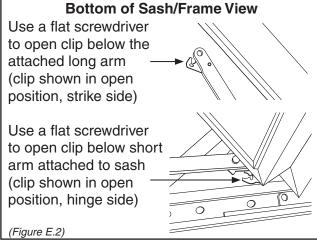
For sash removal, unlock and open sash.
